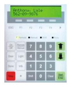
When any of the safety systems are activated causing the machine to stop, the console displays a text message identifying the safety breach.
